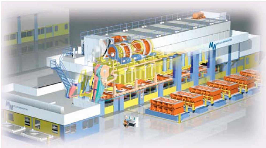
Virtual Reality: Vacuum Transfer Press at 95,000 kN for Automobile Body Parts
