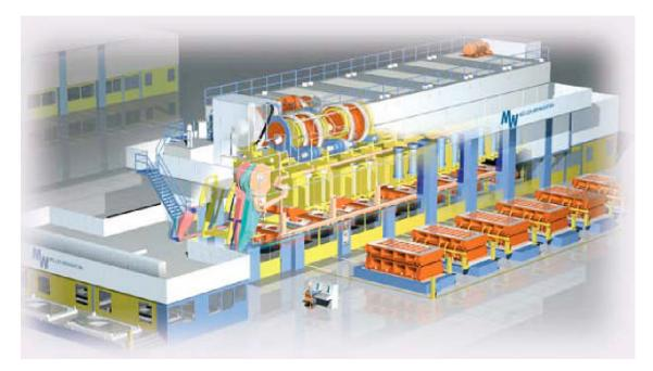
Virtual Reality: Vacuum Transfer Press at 95,000 kN for Automobile Body Parts
