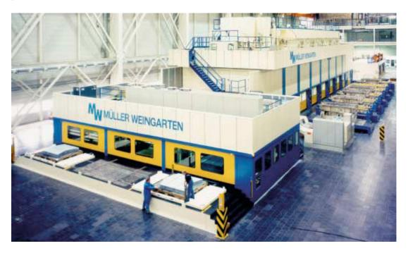
Vacuum Transfer Press for Large-Surface Automobile Body Parts
