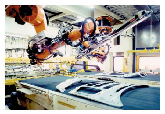
Robot Removes Part from a Large-Format Transfer Press
